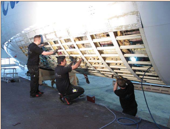
Technicians replacing the covering during a repair of a Boeing 737
